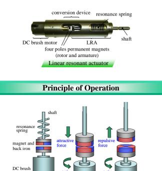
The armature moves linearly in the direction of z-axis as the attractive and repulsive force acts on the armature according to the rotation of the rotor. Because the armature is restricted to linear motion by the sliding guide, it reciprocates twice while the rotor goes round.
