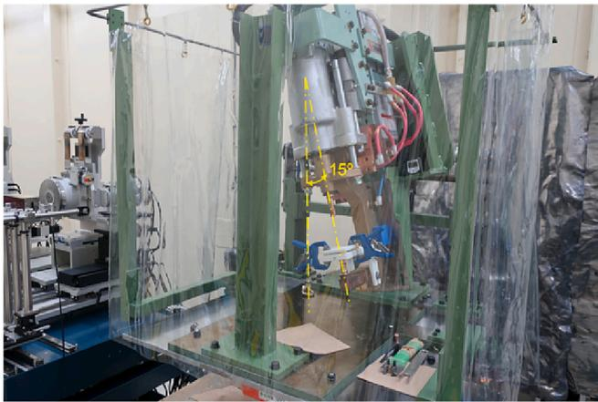
Fig. 1. Photograph of tilted welding equipment.
